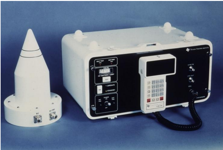
Figure 12: TI-4100 GPS receiver, used in the late 1980s. This box weighed ~80lbs and could track 5 satellites. (Courtesy GPS history website)
