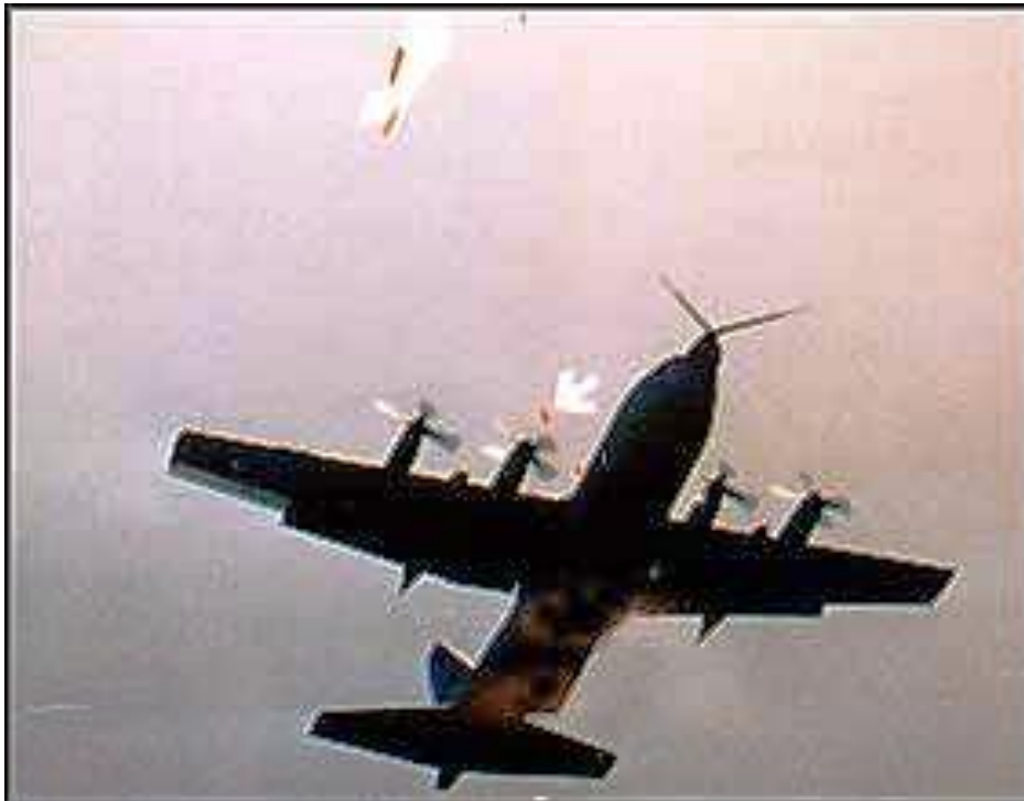
Figure 5: The Fulton "Sky Hook" system in operation. The aircraft catches the balloon cable with the Y-antenna at its nose, and the person being rescued is then winched into the cargo hold. In this photo the balloon appears to be just above the top edge of the photo (Courtesy C130 Sky Hook web site)
